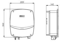
Figure 3.2 Dimensions of R5-0.7K/1K/1.5K/2K/2.5K/3K-S1-15
