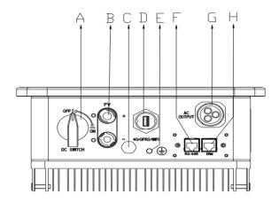
Figure 5.2 Electrical interface of R5-0.7K/1K/1.5K/2K/2.5K/3K-S1-15
