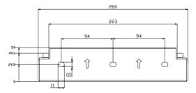
Figure 4.3 Dimensions of rear panel of R5-0.7K/1K/1.5K/2K/2.5K/3K-S1 R5-0.7K/1K/1.5K/2K/2.5K/3K-S1-15
