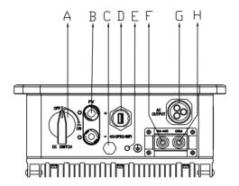
Figure 5.1 Electrical interface of R5-0.7K/1K/1.5K/2K/2.5K/3K-S1
