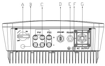
Figure 5.4 Electrical interface of R5-7K/8K-S2
