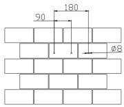
Figure 4.6 Drill holes' dimensions of R5-0.7K/1K/1.5K/2K/2.5K/3K-S1 R5-0.7K/1K/1.5K/2K/2.5K/3K-S1-15
