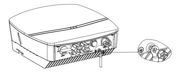
Fig. 5.5 Inverter ground protection
