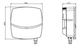
Figure 3.4 Dimensions of R5-7K/8K-S2 R5-7K/8K-S2-15
