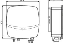
Figure 3.2 Dimensions of R5-0.7K/1K/1.5K/2K/2.5K/3K-S1
