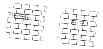
Figure 4.8 Mount the rear panel of R5-0.7K-3K-S1/R5-0.7K-3K-S1-15
