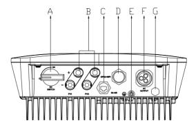
Figure 5.3 Electrical interface of R5-3K/3.6K/4K/5K/6K-S2
